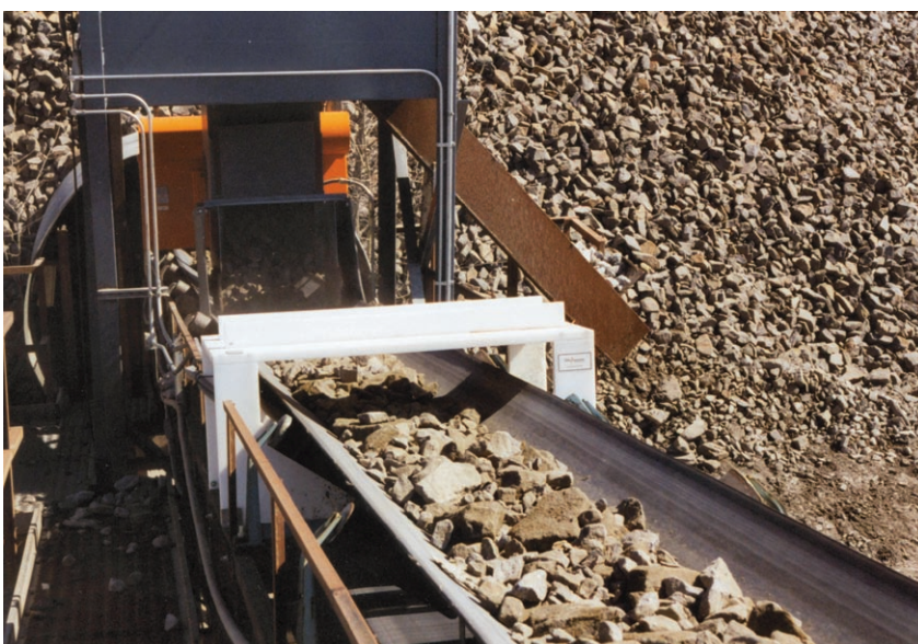
Figure 3. Eriez Model Metalarm metal detector. The conveyor belt runs between an embedded transmitter and a receiver coil.
