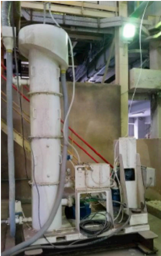
Figure 3: An isometric of the 0.5 metre column that was used to conduct this plant trial. These units can be brought around the world with an experienced Eriez engineer to benchmark or evaluate column performance.
