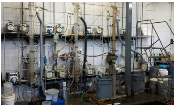
Figure 1: The lab columns used for the reverse flotation of this phosphate ore. Also shown here are the mixing tanks and metering pumps for each of the three conditioning reagents.
